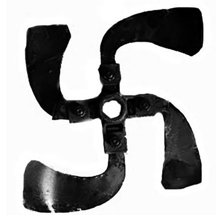
图 5 普通培土刀 Fig.5 Common earthwork knife
