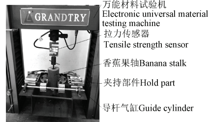
b. 当量摩擦力测量试验图 b. Spot diagram of equivalent friction measuring
