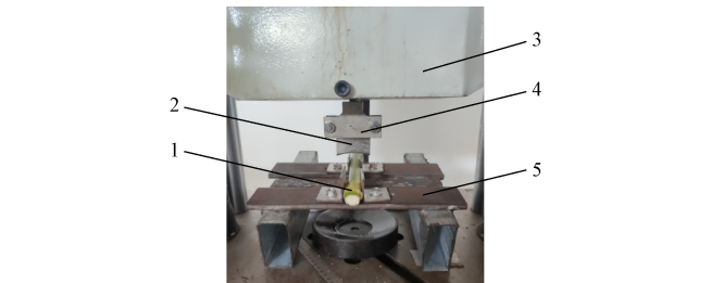
1.玉米秸秆 2.试验刀片 3.WEW-600D 型万能试验机 4.刀片夹具 5.秸秆夹具 1.Corn stalk 2.Test blade 3.WEW-600D universal testing machine 4.Blade clamp 5.Stalk clamp
