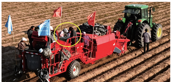
a. 图像采集装置安装位置示意图 a. Schematic diagram of the installation position of the image acquisition device
