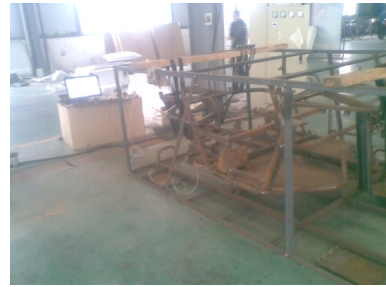
图 2 机架模态试验现场 Fig.2 Modal experimental diagram of sprayer frame
