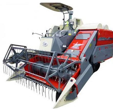
图3 双滚筒联合收割机 Fig. 3 Double Drums Combine Harvester
